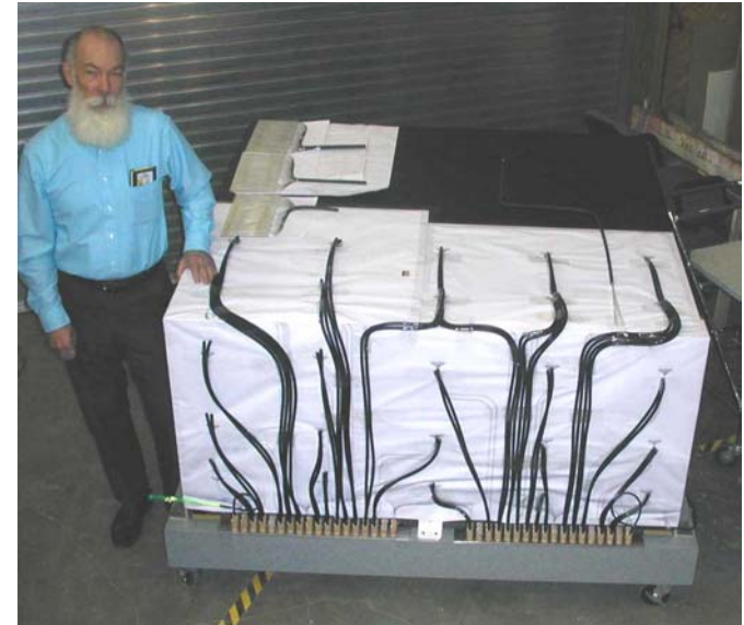
Full-scale mock-up of ACD being used for tile placement and fiber routing
